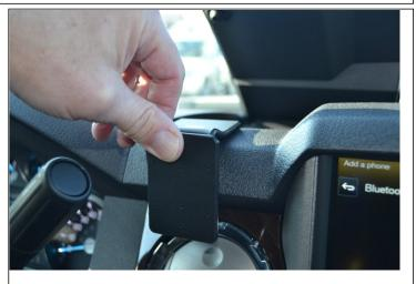
2. Press back on the upper part of the ProClip until the J-shaped angled edge on the top hooks over the dash edge where the dash top door is open.
