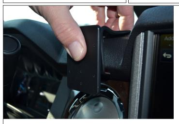
1. Open the door on top of the dash. Peel off the cover of adhesive tape on the ProClip. Place the ProClip in your hand so the ProClip label (sticker) is in an upright position, or if vertically positioned; the P in ProClip is at the top.
