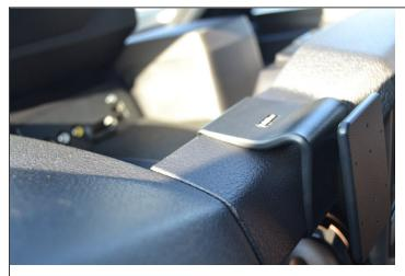
3. Make certain the ProClip goes into the seam between the dash top and the inside tray of the box. The door on top of the dash should close easily.
